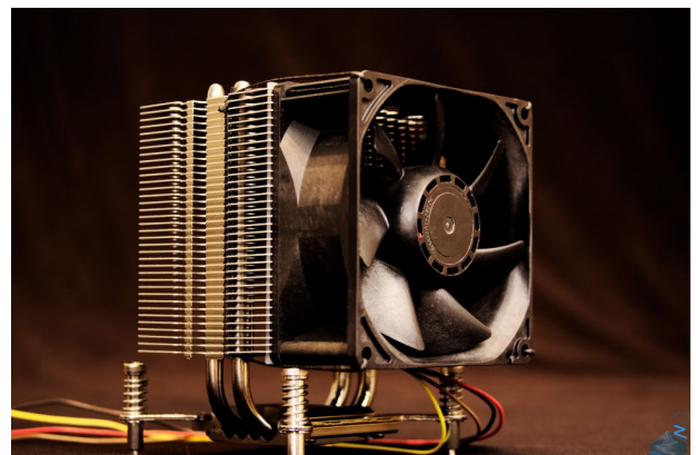
Figure 2.9: The San Ace fan mounted on Noctua heatsink.
