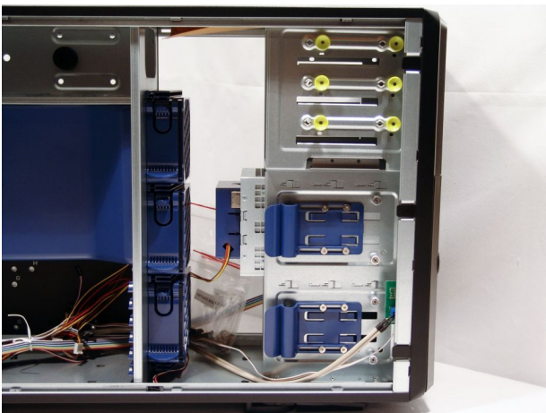
Figure 2.65: Stock configuration. The blue cages can be easily swapped out if needed... (Credit: tweaktown.com [33])
