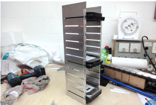
Figure 2.30: Side panels for disk racks completed. Using some old broken HDDs to test fit.
