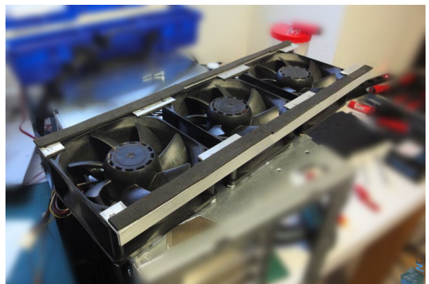
Figure 2.75: Also: Foam between the alu angles and the wall itself.
