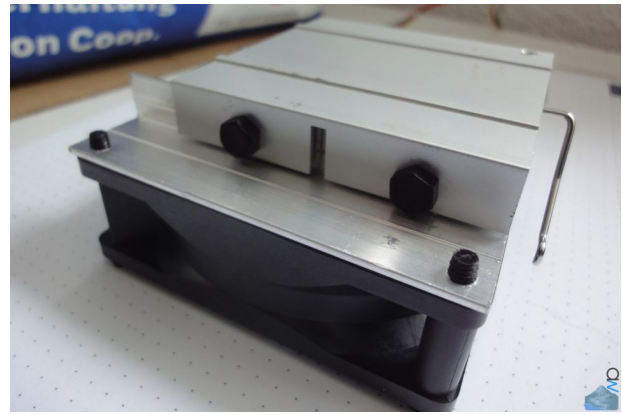
Figure 2.49: The fan is held down by three screws, two in the L piece...
