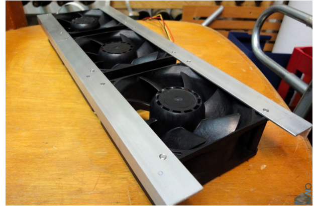
Figure 2.67: M4 screws and alu profiles.
