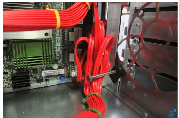
Figure 2.94: The bottom controller had a bit more extra cable length to hide, so that part is a bit messier.
