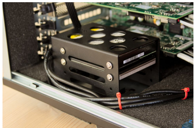
Figure 3.2: That Caselabs drive cage I mentioned, the top drive is the WD Velociraptor.
