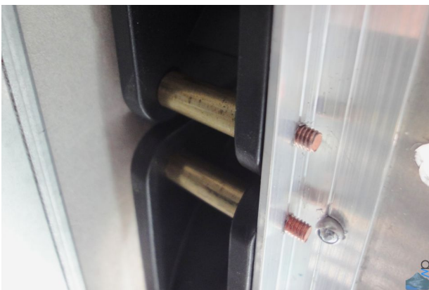
Figure 2.54: Closeup of the brass bushings. Works nicely.
