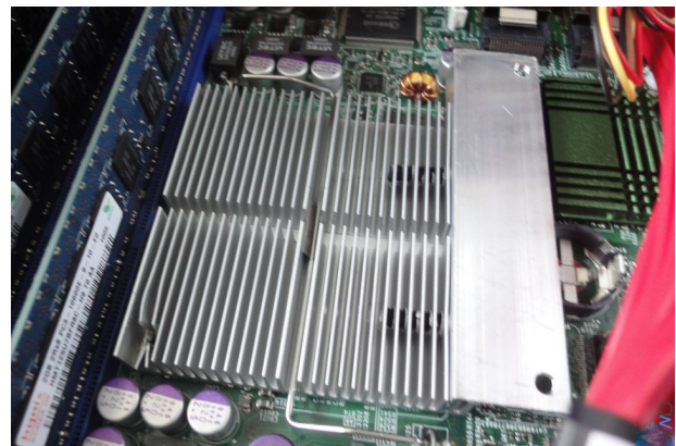
Figure 2.52: For mounting it on the M/B, it needs to be mounted first without the fan...
