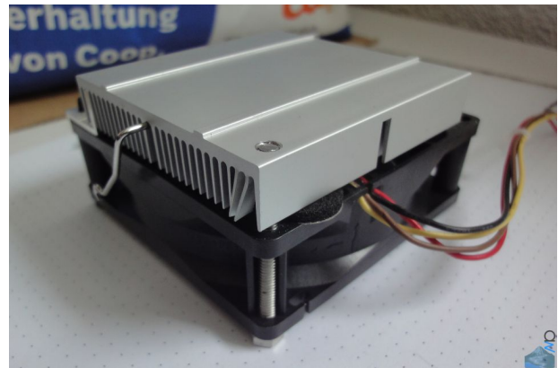
Figure 2.50: ... and one in the corner of the heatsink itself. Some fins are bent from the drilling.
