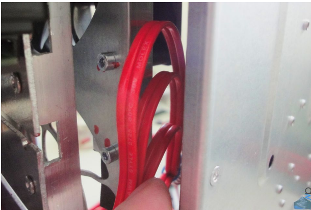
Figure 2.91: Loop of for the topmost cable loom.
