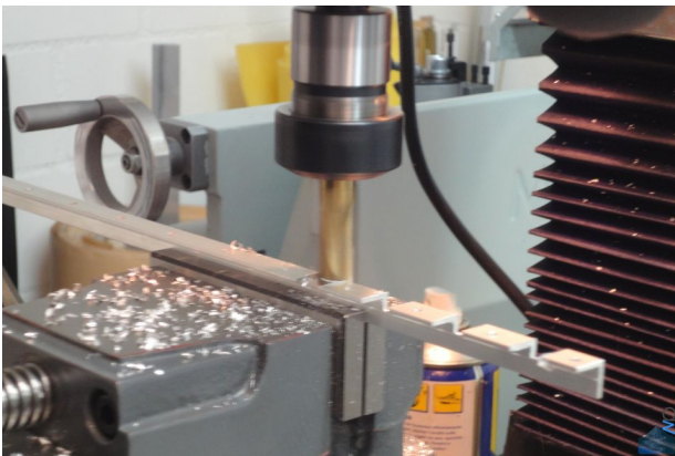
Figure 2.29: Milling out the slots for the screwheads.
