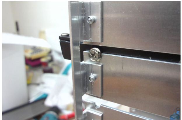
Figure 2.33: A closeup of the rails for the HDDs
